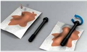
**9.** Lightly lubricate the bolt thread and the bottom of the bolt head by applying a small quantity of oil to a rag and rotating the bolt in the oily rag.
