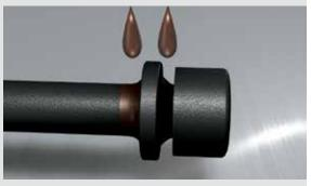
**10.** If the manufacturer specifies the use of a washer, lightly lubricate both sides.
