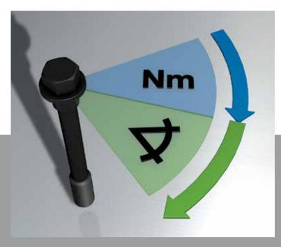
Torque-angle method using pretorque and tightening angle.
