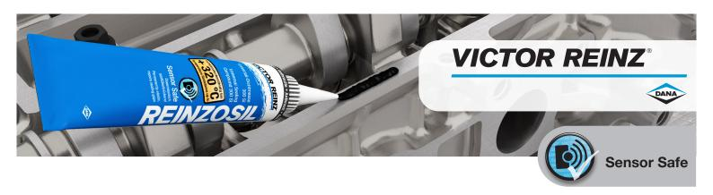
Processing temperature lies between +5 °C and +40 °C. Depending on temperature and humidity, a skin develops after 5 to 12 minutes. The full curing time depends mainly on the relative air humidity (RH) and room temperature, as well as on the thickness (gap height) and width of the applied layer.
