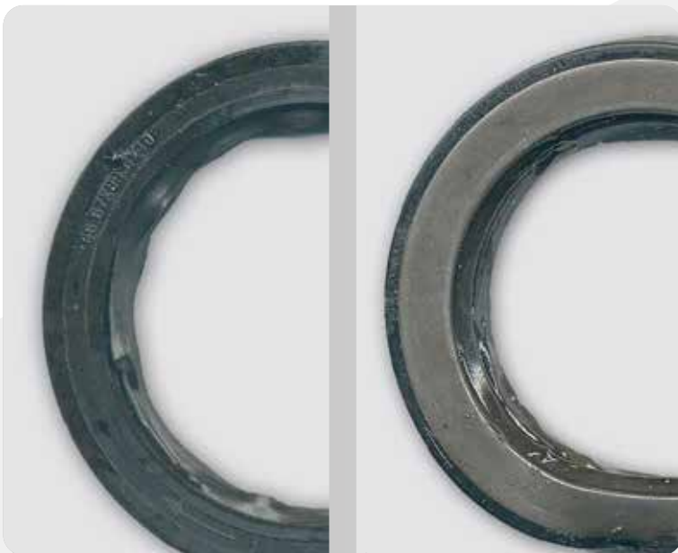
▲ Damaged PTFE sealing lip as the cause of failure.
